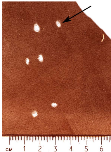
Damage in leather made from hide of cow that had boophilid infestation. The white areas that have not taken up the dye were feeding sites of the ticks.
