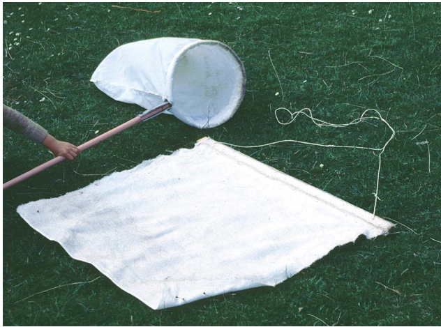
Cloth drag (bottom) and sweep net (top). The cloth drag is 1 metre square.
